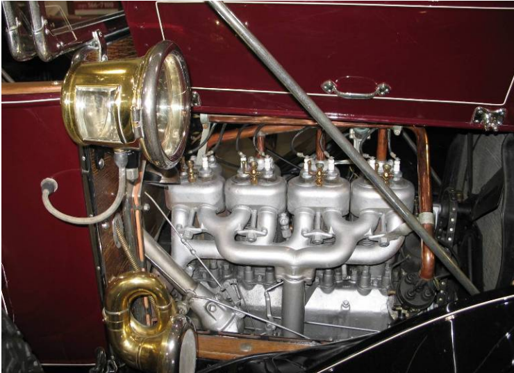
Original 4-cylinder engine displaces 286 cubic inches and produces 40 hp; note the engine compartment is well-detailed and the copper water jackets are a real eye-catcher
