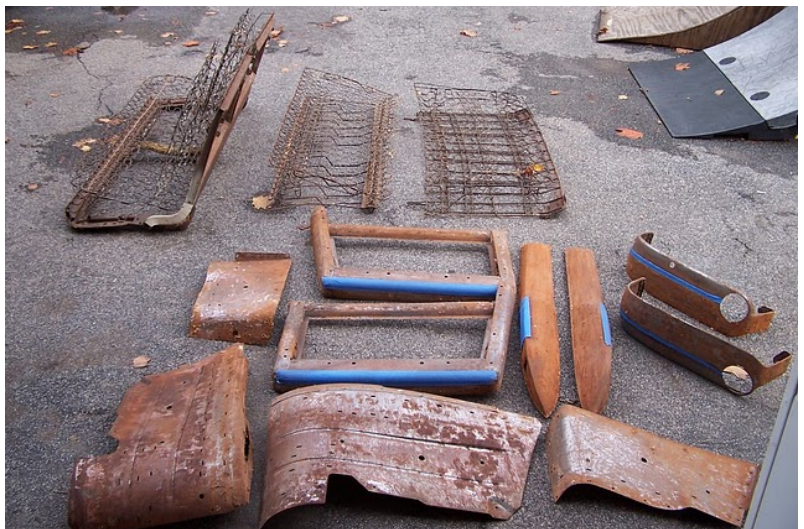
Stripped down interior parts waiting to be blasted and painted before going to the interior shop
