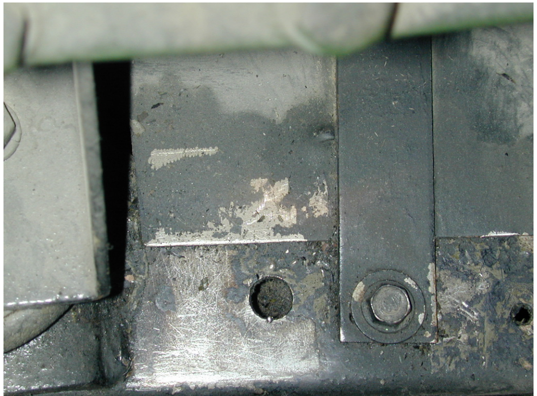
Photo showing where the car's hard-to-find vehicle identification number (VIN) had been crudely filed off the metal chassis
