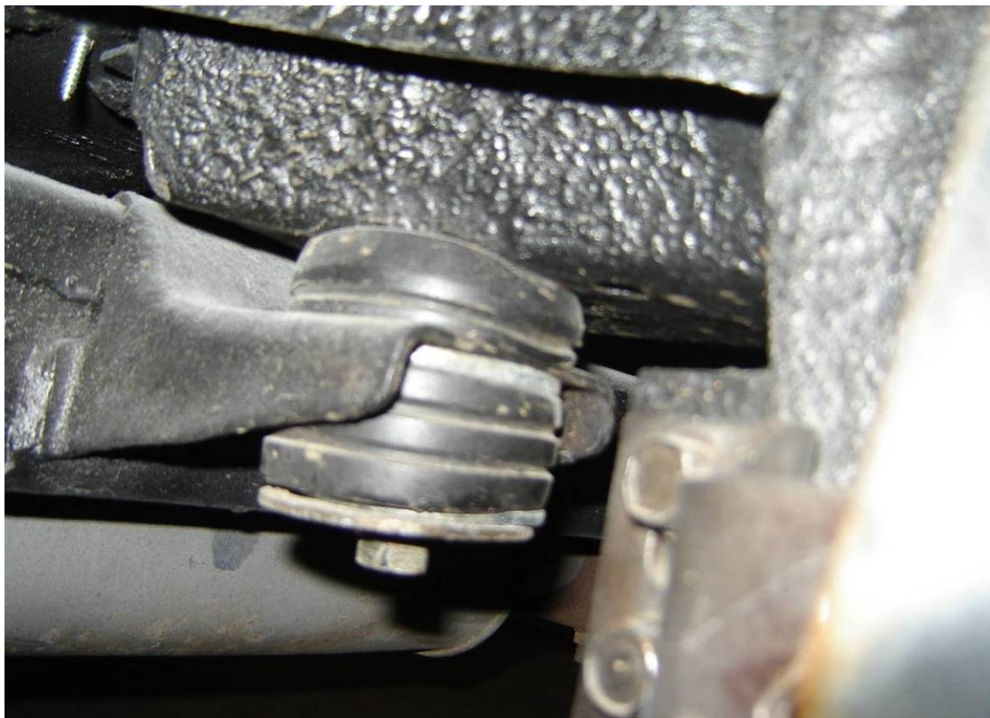
Mission accomplished: replaced bushing
