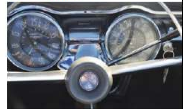
BELOW: When the mileage of Le Mans No. 4 reached 7769 miles (sometime before September 1958), Cadillac's garage lowered the car's steering column by 1-1/2 in. for original owner James E. Goodman, whose initials are engraved in the steering wheel hub.
