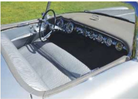
ABOVE: Gauges were spread across the width of each Le Mans ' instrument panel. The original seat upholstery of each Le Mans originally included a Cadillac V and crest in the center of the seat back rest, but that detail was eliminated from Le Mans No. 4 at some point in its past.
