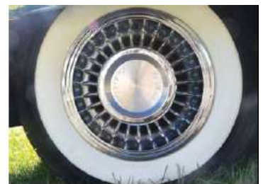
ABOVE: The Le Mans wheels predicted the Sabre-spoke wheel first used in production during 1955.
