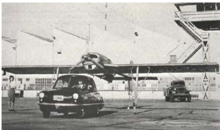
Theodore Hall's Convaircar would rent its wings at airport franchise, then back into position for hookup.
