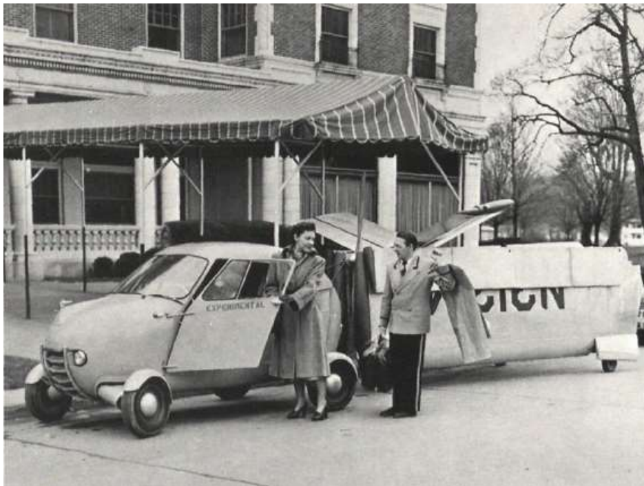
Taylor's wife got into prototype of Aerocar I after hotel stopover in '50s. Folded wings and tail were towed in trailer.
