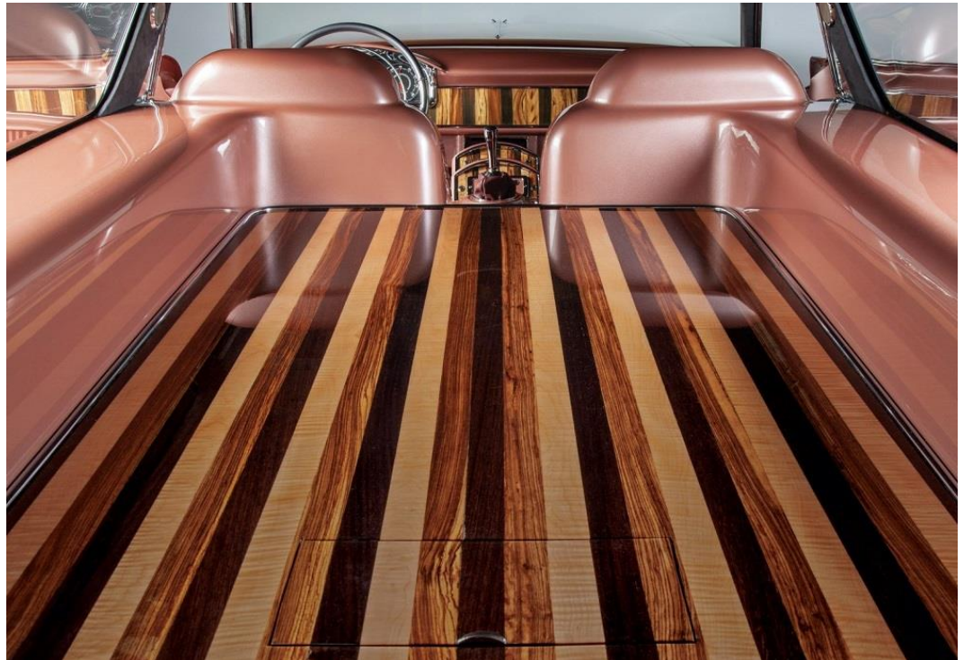
Except for the powertrain, everything under CadMad's floor was made from scratch. The cargo area was finished to glass-like perfection with automotive clearcoat, the dash painted to match.
