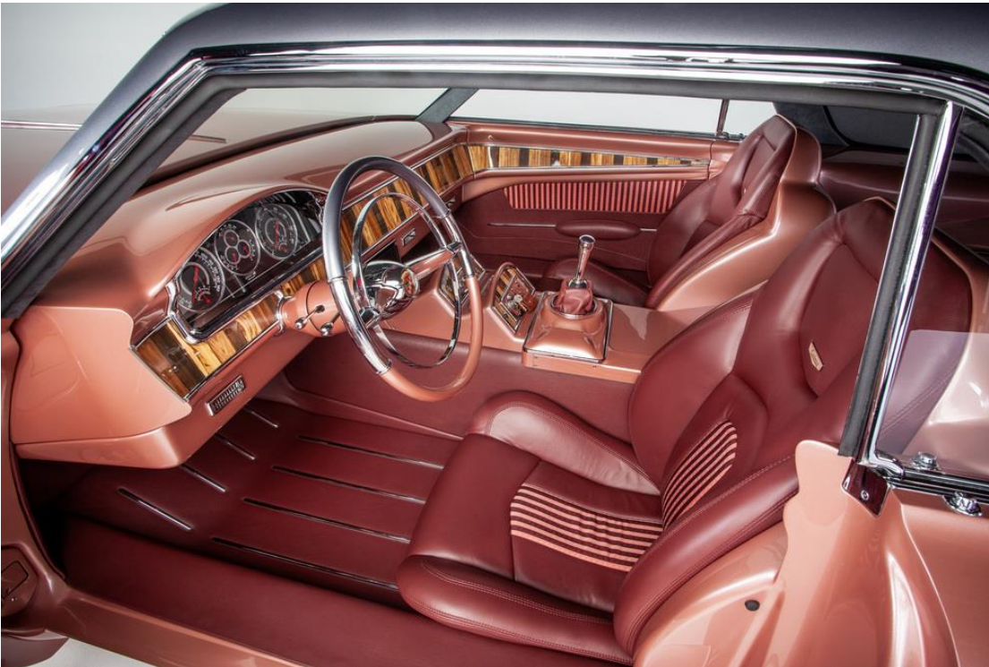
A paddle-shift idea failed just months before the show, so the Quintals quickly made an elegant console shifter.
