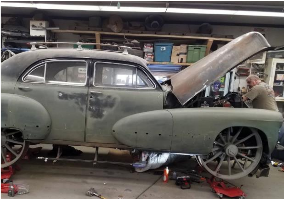
Jack Sanford working under the car while Bryan Totten replaces the original fuel pump Photo by the West Virginia Railroad Museum
