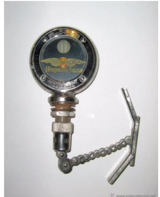
How another style of Moto-Meter lock attached to a Moto-Meter. When unfolded below the filler neck, the hinged arms of the lock prevent removal of the Moto-Meter.
