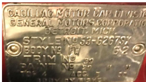
Body Tag Attached to Firewall of Eldorado #62 with Correct Type Rivets
