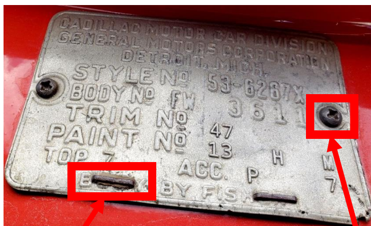
Body Tag on Convertible Cowl with Staples and Correct Screws Courtesy Hemmings Auctions
