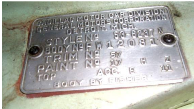
Red Primer Showing Around Edges of Body Tag Posted on the CLC Forum by Paul Allen
