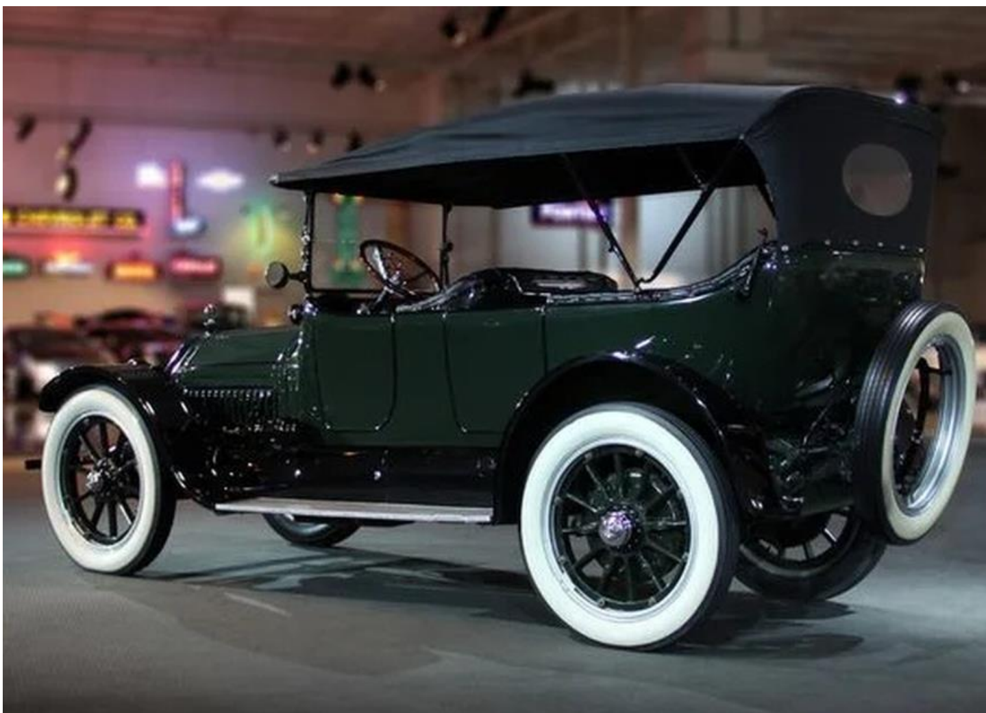
1915 Cadillac Type 51: the first car to use a key ignition, three-pedal layout, and center-mounted gears
