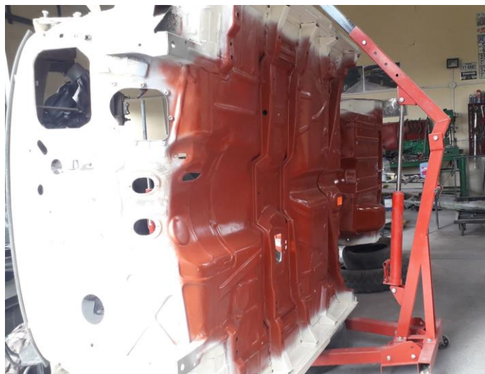
Underside: Above, as received in Georgia Below, after de-rusting
