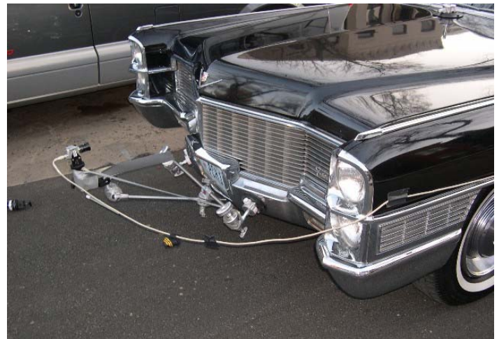
Camera mounted to the front of the car
