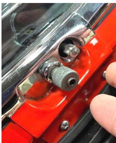
FW 8, old style escutcheon; screws exposed for photo
