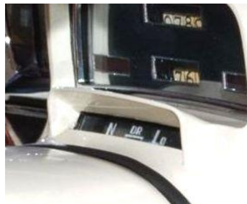
Right: Later shift quadrant bezel with lip on top to block reflections
