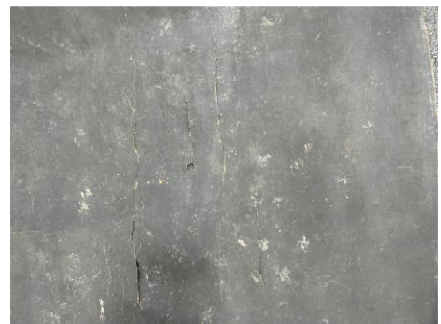
Photo left shows the old top material removed from the car's roof. The hole for the vent and the screw holes for its mounting flange are readily visible. Some of the tears in the brittle, original material can be seen in this image below.
