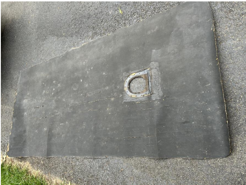
Photo left shows the old top material removed from the car's roof. The hole for the vent and the screw holes for its mounting flange are readily visible. Some of the tears in the brittle, original material can be seen in this image below.
