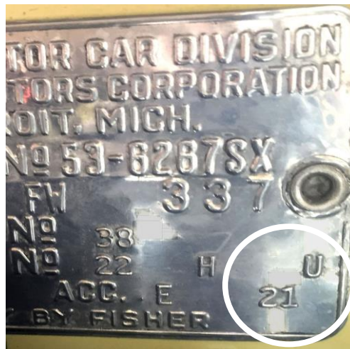
Eldorado FW 337, after 10 Dec 52 U = interior paint code for red 21 = date code for day of month
